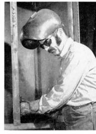
DOUBLE PROTECTION in the form of safety goggles and steel welding hood is worn by Samuel C. Waldorf, are welder in 2123-4.
